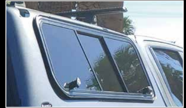
Optional side Window with Slider provides ventilation without opening the entire Window
