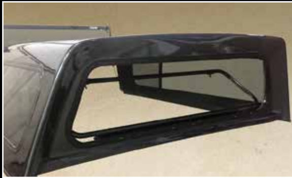
Optional cap tilt down Hinged Front Window allows access to wash back window of truck
